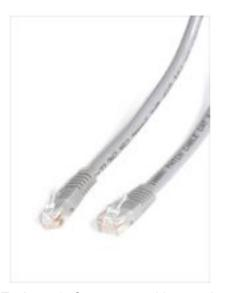
StarTech.com's Category 6 cables are the perfect way to connect your workspace's emerging gigabit networks. Category 6 cables improve upon the Category 5e specification by providing twice the available bandwidth (up to 250Mhz), and a signal-to-noise margin improvement that is sixteen times (12dB) better than that provided by Cat 5e.<br/>
