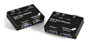
The Converge A/V VGA over Cat5 video extender allows up to 4 (2 local and 2 remote) monitors to be connected to a single PC. The video signal is sent to remote monitors over standard 4 pair Category 5 UTP cable using RJ45 connectors and supports distances of up to 150m / 500ft. The ST121UTP is an out-of-the box solution that includes both the local transmitter and remote reciever.
