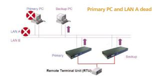
**Host redundant:** CN2610 can provide the synchronous communication ability to establish connections to Primary PC and Backup PC at the same time. Once Primary PC is dead backup PC will take over the control immediately.
