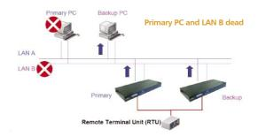
**Data acquisition redundant:** CN2610 DRDAS mode plays the role to communicate with up to 4 IP addresses. In the previous page's picture, CN2610 receive the RTU's data from serial port, and send the data to 4 IP addresses in 2 PC in the different LAN. 1 of the 4 IP address is the primary IP to send the down stream data to RTU and the other 3 IP cannot send data to RTU. Via this architecture, if Primary PC, LAN B and Primary CN2610 crash at the same time, the system still work without problem.
