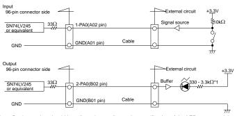
Resistor value should be adjusted according to the specification of the LED to use and the desired intensity level.
