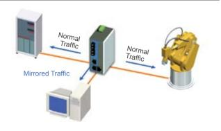
devices almost instantaneously when exceptions occur. The traditional way of determining device status is to poll devices periodically, but this is not "real-time" enough, and is not very efficient. Warning messages must be actively triggered by events. To take care of these requirements, industrial Ethernet Switches need features such as:
