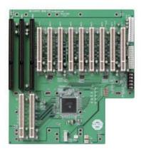
BPM-1111 is the Backplane board which have the 2 PICMG (PICMG+ PICMG/PCI) + 8 PCI + 1 ISA slots. The Backplane board have two CPU board(SBC) PICMG Bus slots(PICMG1 and PICMG2) and eight PCI Bus slots(PCI2 - PCI9) and one ISA Bus slot(ISA1). PICMG2 and PCI1 is shared Bus slot.
