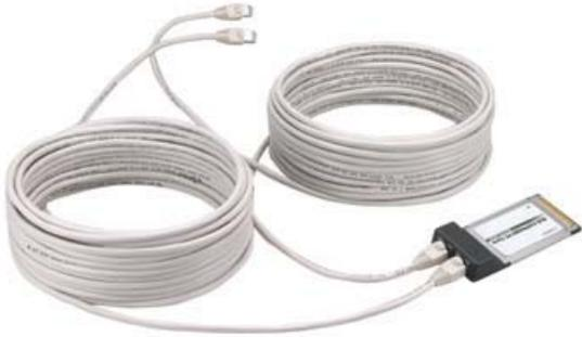
The EAD(CB)SF is an expansion adapter that connects the optional expansion chassis [ECH(PCI)SF] to a PC to extend a CardBus compliant PC Card slot in the PC, thereby providing additional PCI bus slots. The expansion adapter can connect the expansion chassis to the PC over a distance of up to 12m.
