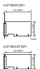
The standard outside dimension (L) is the distance from the end of the board to the outer surface of the slot cover.
