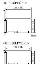
The standard outside dimension (L) is the distance from the end of the board to the outer surface of the slot cover.
