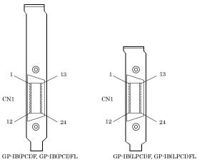
On-board connector : 555139-1(AMP) Applicable connector(cable): GPIB cable(IEEE-488 rated)
