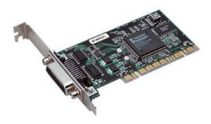
High Speed & Function IEEE-488.2 I/F Board for Low Profile PCI
