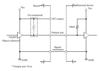
The output circuit of interface is illustrated in Figure. Signal outputs are open-collector outputs; individual output signals are sent to the external device as active low signals. Note that each signal output must be pulled up at the external device as it is not pulled up internally.
