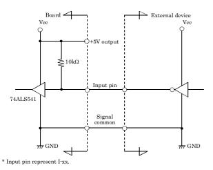
The input circuit of interface is illustrated in Figure.
