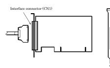
Connector used 50-Pin Mini-Ribbon connector 10250-52A2JL[mfd.by 3M]
