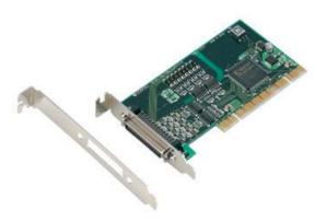
This board is a PCI-compliant interface board for input/output of digital signals.
