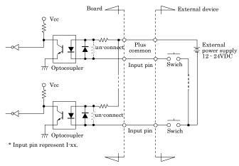
The input circuit of interface is illustrated in Figure 3.3.
