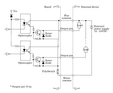
The output circuit of interface is illustrated in Figure 3.5. The signal output section is an opto-coupler isolated, open-collector output (current sink type). Driving the output section requires an external power supply.
