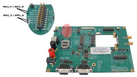
Figure 8-1: Mini Card Dev Kit showing MIC/SPK pins.
