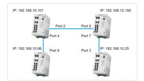
JetNet 5310G supports topology discovery or LLDP (IEEE 802.1AB Link Layer Discovery Protocol) function that can help users to discover multi-vendor's network devices on the same segment by an NMS system which supports LLDP function. With LLDP function, NMS can easily maintain the topology map, display port ID, port description, system description, VLAN ID and so on. Once a link failure happens, the topology changed
