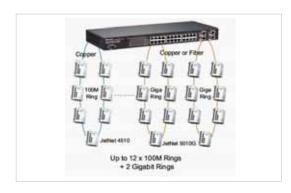
The JetNet 5728G series supports the new generation ring technology – MSR<sup>TM</sup> which includes various new technologies for redundancy applications and structures of different networks. The PoE switch allows to aggregate up to 14 Rapid Super Rings, including 12 Fast Ethernet plus 2 gigabit Ethernet Rings. With the MSR<sup>TM</sup> technology, a node can be configured to multiple rings with the failover time in as little as 5ms, and zero-second of restoration time.
