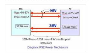
JetNet 5728G series implements the 2-event and Link Layer Discovery Protocol (LLDP) PoE into the system for efficient power budget negotiation between PSE and PD devices. The LLDP packet provides smart power budget control behavior to fulfill the needs of higher end setups requiring exact high power delivery. By using the ongoing dynamic re-negotiation function of the IEEE802.3at LLDP PoE, the JetNet 5728G series can perform more intelligently by dynamically reallocating power to the PDs.
