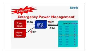
power higher and lower wattage devices according to user-definable parameters such as maximum available power, port priority (critical, high, low), and maximum allowable power per port.
