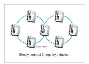
directions. In addition to extensibility, MultiRing<sup>TM</sup> has great diversity of various ring technologies. With MultiRing<sup>TM</sup> enabled, a device can connect  $RSR^{TM}$  rings, TrunkRing<sup>TM</sup> and a ring of Super Ring together. Which provides extensibility to new technologies while keeping the great backward compatibility.
