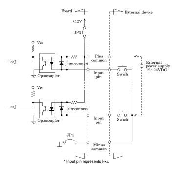
The input circuits of interface blocks of the DI-32B-PE are illustrated above. Connect the input signals to a device which can be current-driven, such as a switch or transistor output device.
