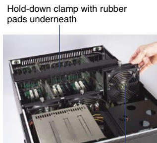
Three 114 CFM hot-swappable cooling fans
